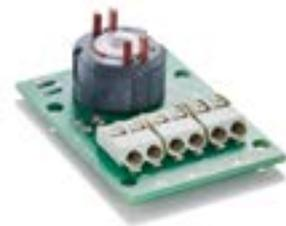
Contact module for standard actuators
